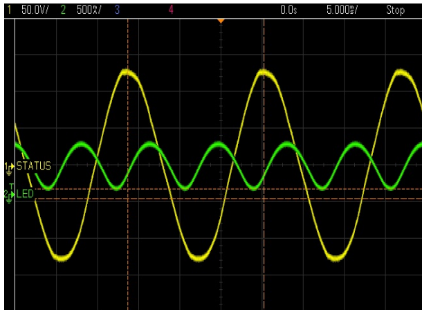
Figure 12. Input AC voltage vs. output current
