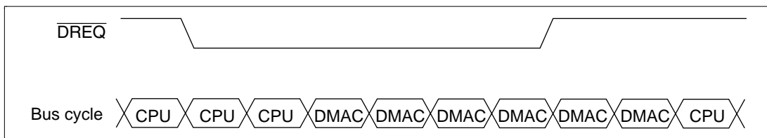
Figure 11.13 DMA Transfer Example in the Burst Mode
