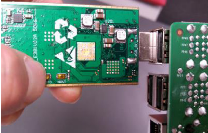
Figure 14: STM32 MCU Boot0 Button
