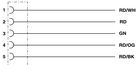
Contact assignment of 7/8" plugs/sockets, cable type 420
