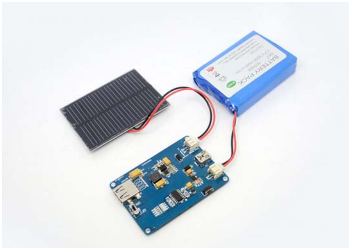
Charge Lithium Polymer Battery through solar power
