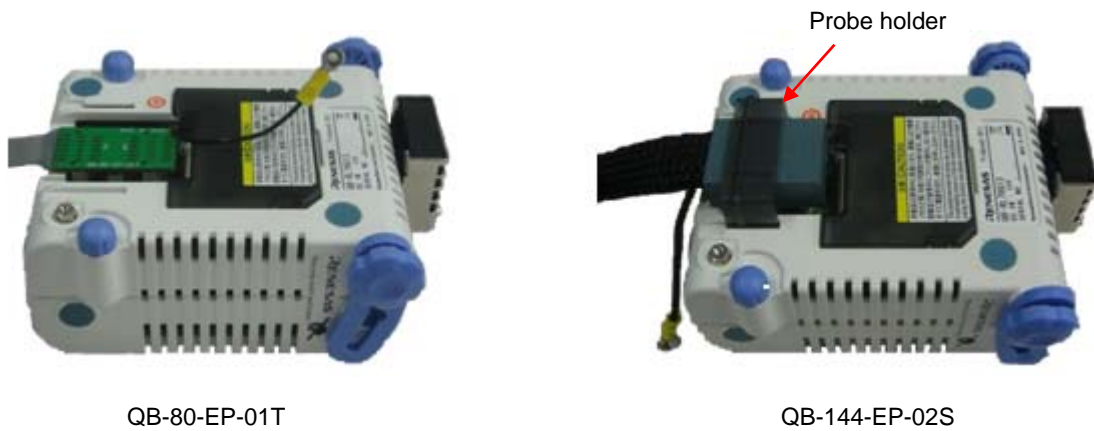
Figure 2-7 Connect the QB-RL78G13 to the probe
