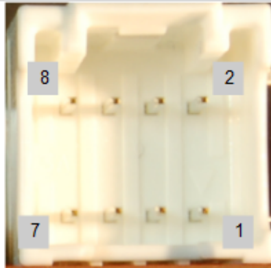
Figure 7. Main Power Connector Pin Orientation
