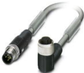
Bus system cable, CANopen®, 5-position, PUR halogen-free, Gray RAL 7001, shielded, Plug straight M12-SPEEDCON, A-coded, on Socket angled M12-SPEEDCON, A-coded, Cable length: 20 m
