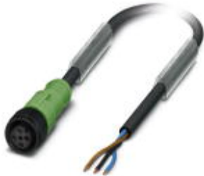
Sensor/Actuator cable, 3-position, PUR halogen-free, Black-gray RAL 7021, Free cable end, on Socket straight M12, A-coded, Cable length: 3 m, with plastic knurl
