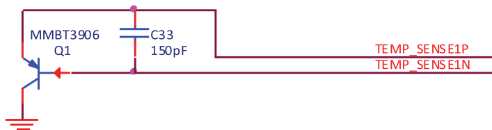
Figure 8.4. PNP Temperature Sensor Circuit
