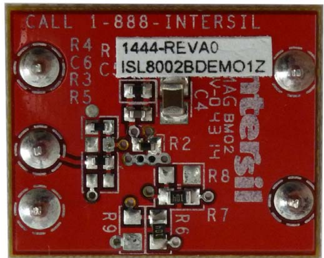
FIGURE 2. ISL8002BDEM01Z BOTTOM SIDE
