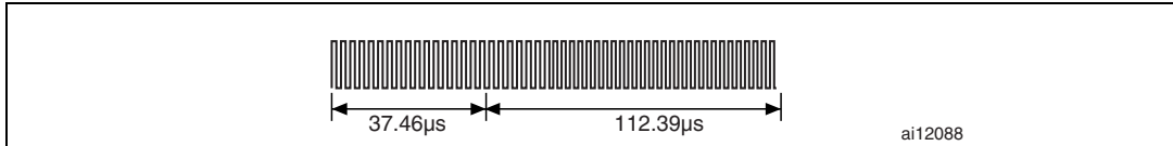
Figure 34. End of frame, high data rate, two subcarriers
