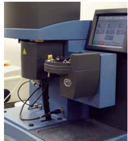
Thermogravimetric Analyzer (TGA) – Measures the stability of our dielectrics at high temperatures, baking the materials at prescribed temperatures and measuring weight loss.
