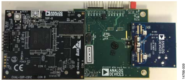
Figure 9. Connecting the ADUX1020-EVALZ-LED Daughterboard
