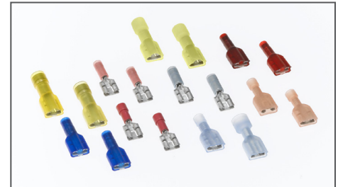
Quixon Fully-Insulated Quick-Disconnect Terminals (Red = 18 to 22 AWG; Blue = 14 to 16 AWG; Yellow = 10 to 12 AWG)
